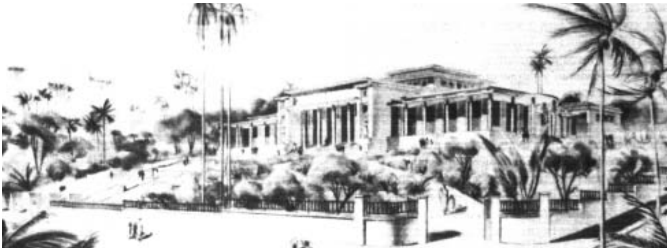
FIGURE 18. Conseil Général Headquarters at Basse Terre. Succession of porticos and peristyles shading the facades enhances the progression onto the core of the building. A square tower culminates at the top of the building, providing ventilation to the different rooms. (Drawing by Ali Tur, in Encyclopédie de l'Architecture: Architecture Coloniale, Guadeloupe: Bâtiments gouvernementaux et communaux, Ali Tur, Paris, Editions Albert Morancé, 1930.)
