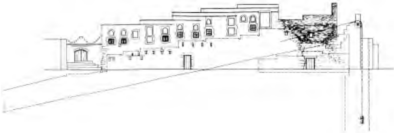
FIGURE 13. (ABOVE) Street elevation of the marna’ (well enclosure) of Talha mosque, ca. 1980. The dashed section lines show the ramp for the animals that operated the pulley, with the well at right. The rooms above housed a Qur’anic school and living quarters for the instructor. Source: R. Lewcock and R.B. Serjeant, Sana’a, An Arabian-Islamic City , 1983. Reprinted by permission of author.
